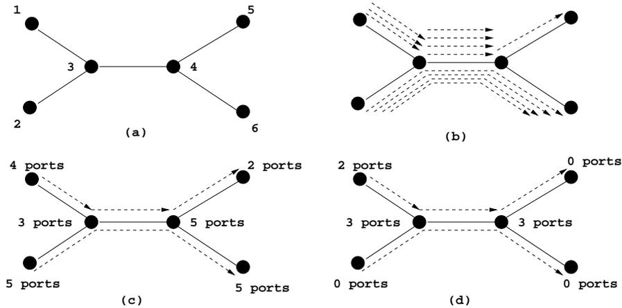
Figure 1.2. (a) Example 6-node physical topology and network state with (b) OC-12 groomer, (c) OC-3 groomer and (d) mixed groomer
